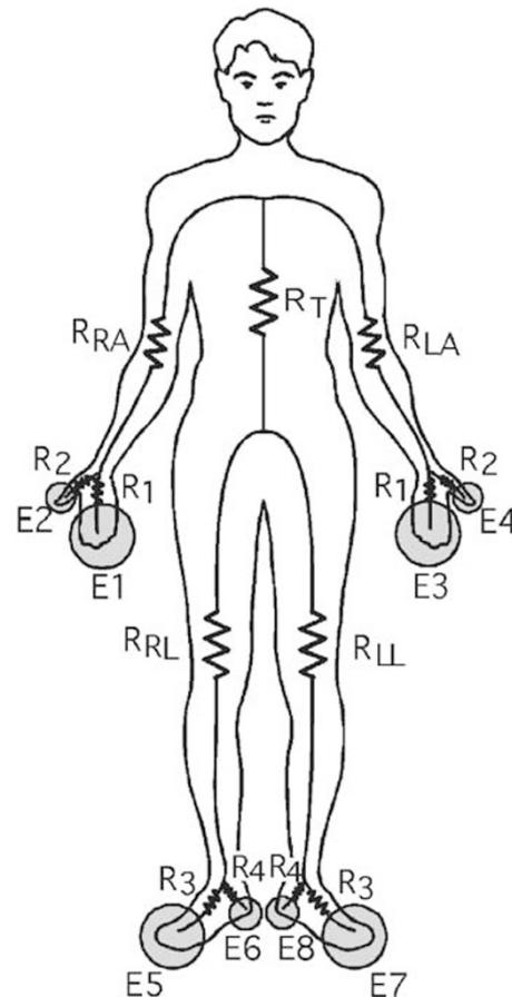
**Figure 1** Measurement pathways of InBody 3.0 (reproduced with permission from Biospace). The subject stands with her or his soles in contact with the foot electrodes and grabs the hand electrodes. Abbreviations: *R<sub>RA</sub>* = resistance of right arm; *R<sub>T</sub>* = resistance of trunk; *R<sub>LA</sub>* = resistance of left arm; *R<sub>RL</sub>* = resistance of right leg; *R<sub>LL</sub>* = resistance of left leg (see text for details).
